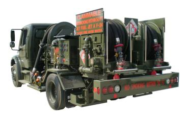
The Isometrics Inc. R-12 is a hydrant dispensing truck intended for refueling a wide variety of aircraft from fighter jets to wide body transport aircraft from Type III hydrant systems.
